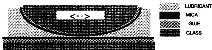
FIGURE 1 Schematic representation of a cross-section of the experiment. The separation of the two mica surfaces is exaggerated. Due to attractive forces the contact point is flattened out. In reality, the ratio between the diameter of the area of contact and the separation of the two mica surfaces is of the order of 10^4 .
